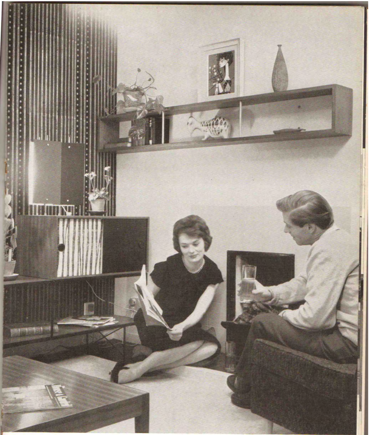
House warming. This tiled fireplace is built into a central core—for a beautifully warm house. Behind the fire (very modern and efficient) is a back boiler with built-in gas ignition. You get piping hot water and a couple of radiators, and a heated towel rail and a warm linen cupboard. A thermostatically controlled immersion heater takes over in summer.
